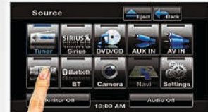
Touch panel controlled GUI provides intuitive access to a multitude of functions while reducing the number of physical buttons.
